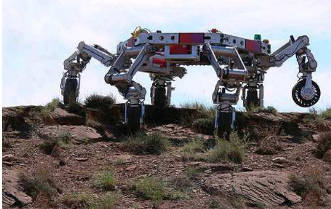
To moonproof rovers such as the cargo-hauling ATHLETE, NASA will have to create tons of simulated lunar dust.
